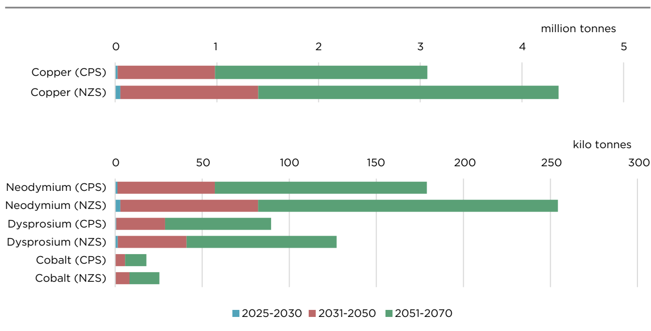
Figure 2.7: EV Motors – Embedded Mineral Requirements
