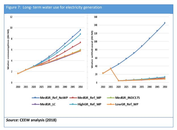
There is some interesting dynamics that need to be highlighted- when older plants move from OTC to CT technology, there is an increase in water consumption. The consumption coefficient of CT technology is higher as compared to the OTC technology. But all the new power plants, have to adhere
