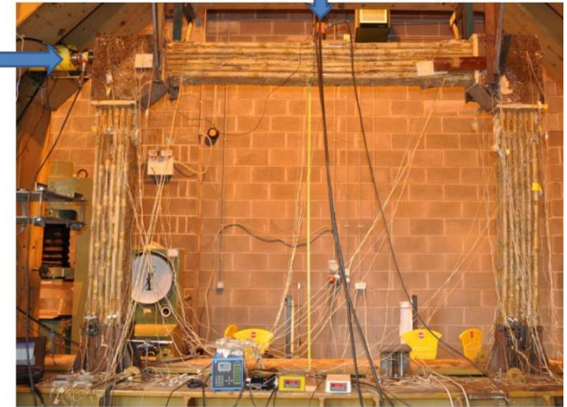
Experimental Setup of 5x6 FRBC portal frame
