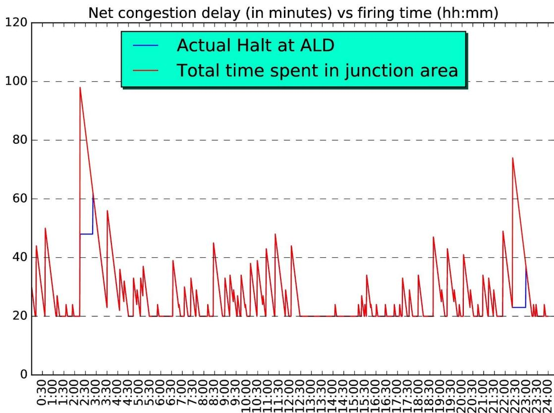
Figure 5.2: Delay experienced by freight trains while entering a junction at various times of the day
