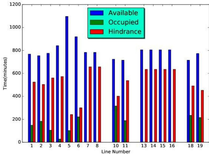
Figure 5.1: Time lost due to hindrances caused due to cross-movements in a junction area: ALD
