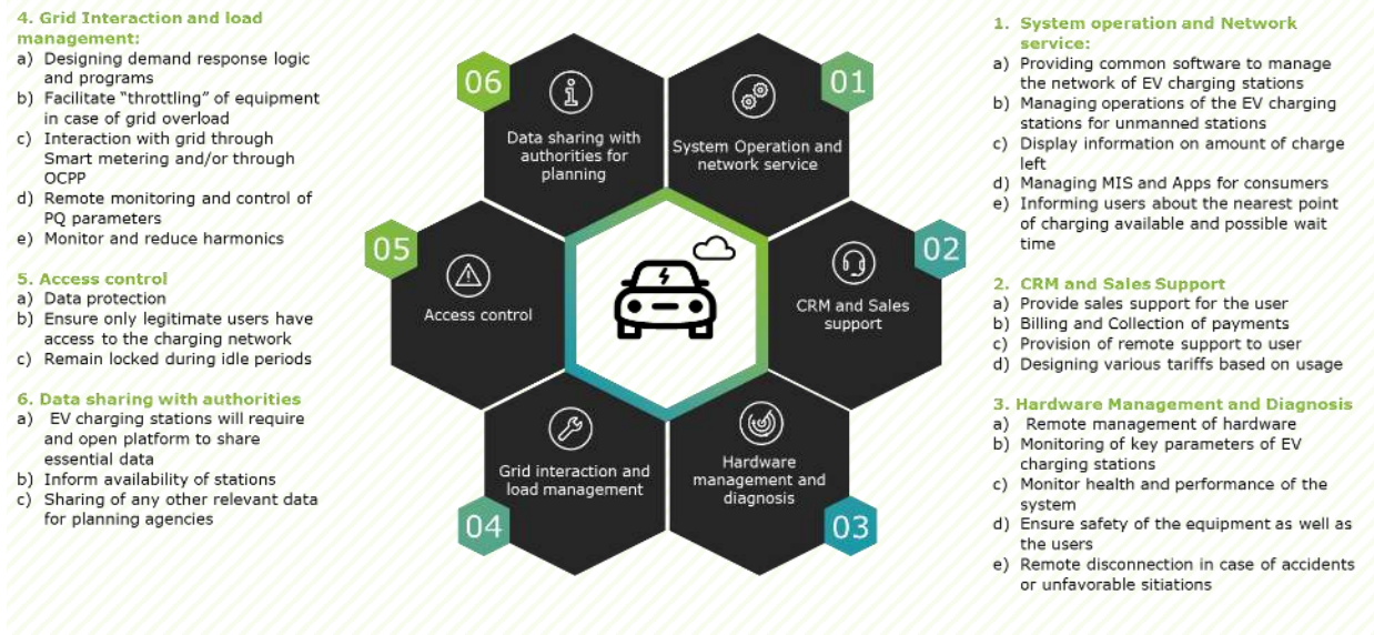
Figure 215 Functions of a network service provider
